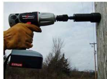
1/2" Sq. Dr. Double Sq. Deep Well — Double Duty • 2 Sockets in 1 • Length: 5"
